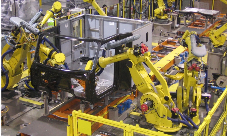
Peterbilt’s Denton, Texas Factory Robotic Cab Assembly Equipment
